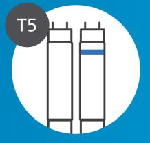
No ring/one ring: Mains (Electro-magnetic ballast or direct mains)
