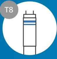
Two rings: HF (High-frequency Electronic ballast)
