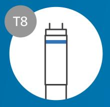
One ring: EM/Mains (Electro-magnetic ballast or direct mains)
